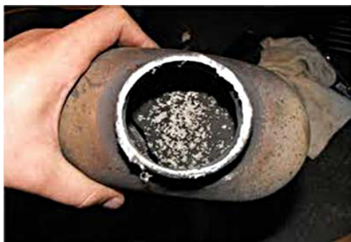
Sealant or coolant clogging
