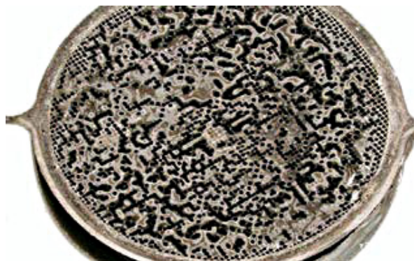
Blockage due to oils or coolant
