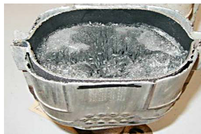
Burning damage due to over fuelling
