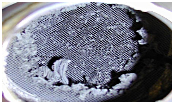
Burning damage due to over fuelling
